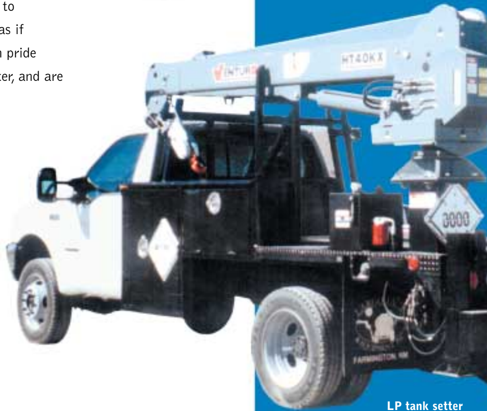
LP tank setter
